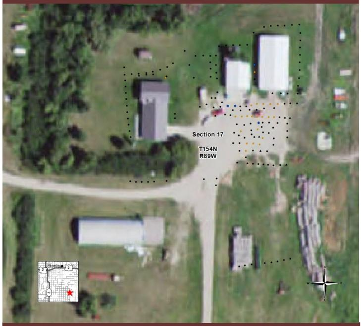
**Shell Lake –Wally Lee Farmstead**. Each dot represents one drill hole. Drilling encountered solid coal at black dots and no coal at black triangles. Grout was pumped into holes at Blue dots and orange dots are holes filled by pumping grout into a different hole.
