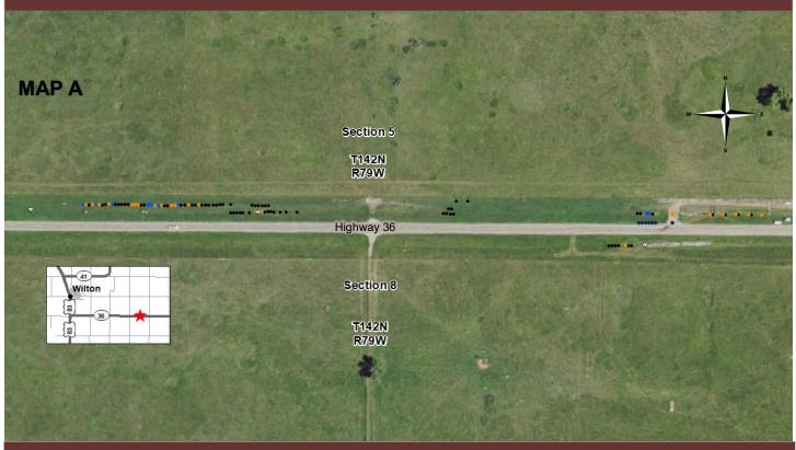
**Maps A & B:** North Dakota Highway 36 runs east and west. Each dot represents one drill hole. Drilling encountered solid coal at **black dots**. Grout was pumped into holes at **Blue dots** and **orange dots** are holes filled by pumping grout into a different hole. **White dots** are core holes.
