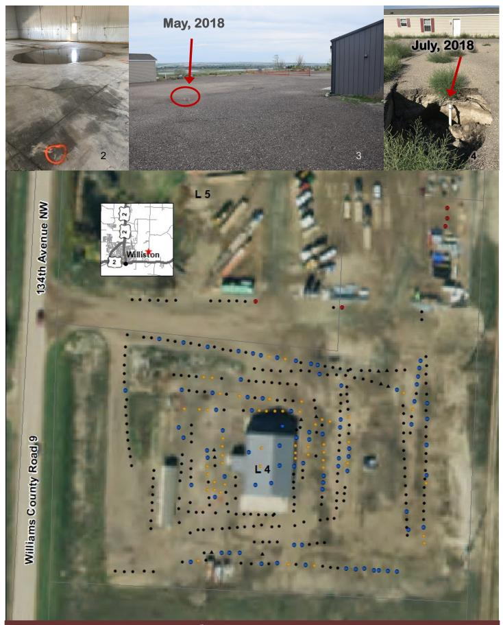
Williams County Road 9, also called 134<sup>th</sup> Avenue NW, runs north and south. Drilling encountered solid coal at black dots and no coal at black triangles. Grout was pumped into holes at Blue dots and orange dots are holes filled by pumping grout into a different hole. Red dots show holes that need grout.
